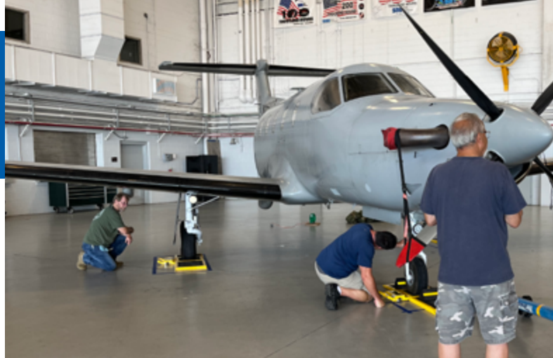
The U-28A being weighed on Intercomp AC15-LP™ Low-Profile Aircraft Scales
