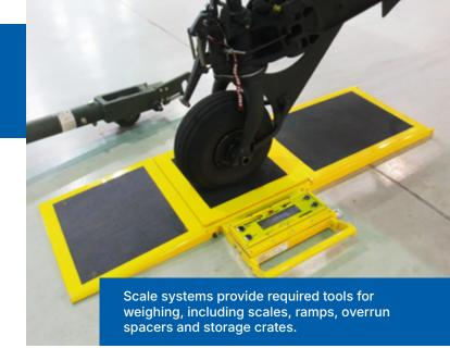
Each eVTOL aircraft is unique, therefore the weighing needs may differ from company to company. Two of Intercomp's eVTOL customers required real-time weight measurement, as well to integrate that data with the vertiports used. Intercomp's <u>AC15-LP™ Low-Profile Aircraft</u> <u>Scales</u> have remedied these challenges.
