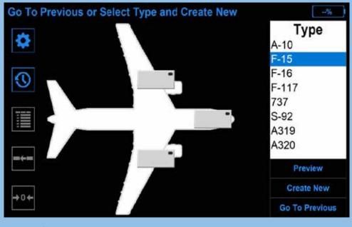
System setup screens show how flexible and powerful the TAC30™ user interface is for users. Customizable data fields, such as user session information for scale operation on a particular day, and/or location and aircraft-specific information can be associated with saved records and included on tickets from the integrated printer
