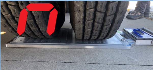
Inner Tire Wheel Weight Displayed
