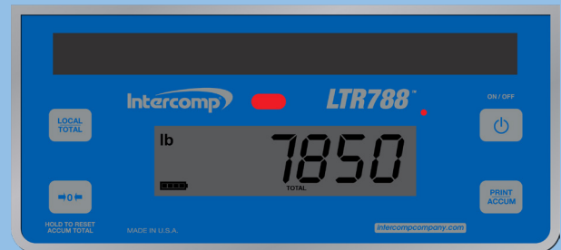
Indicates Total of Both Wheel Weights
