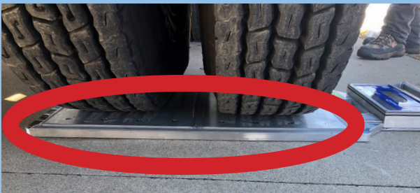
Indicates Total of Both Wheel Weights
