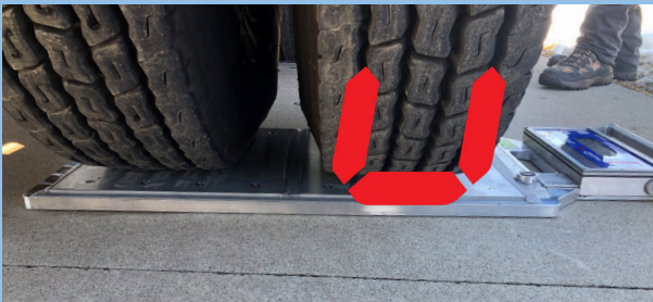
Outer Tire Wheel Weight Displayed
